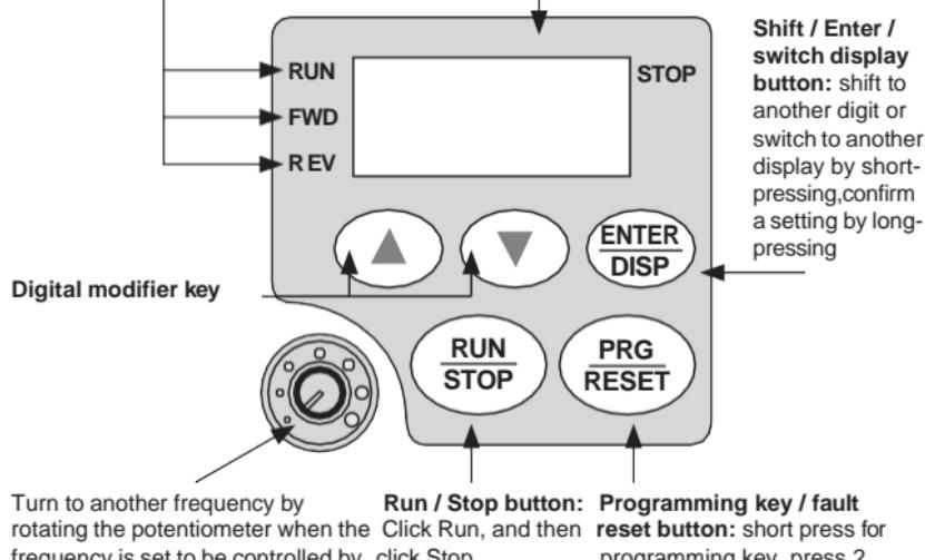
Turn to another frequency by rotating the potentiometer when the frequency is set to be controlled by the manipulator potentiometer
