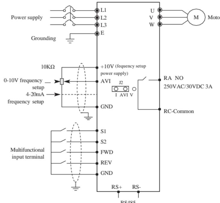
Note: AVI terminals can be used to select an analog voltage input(0-10V) and analog current input (4-20mA ) through the switch J2.
