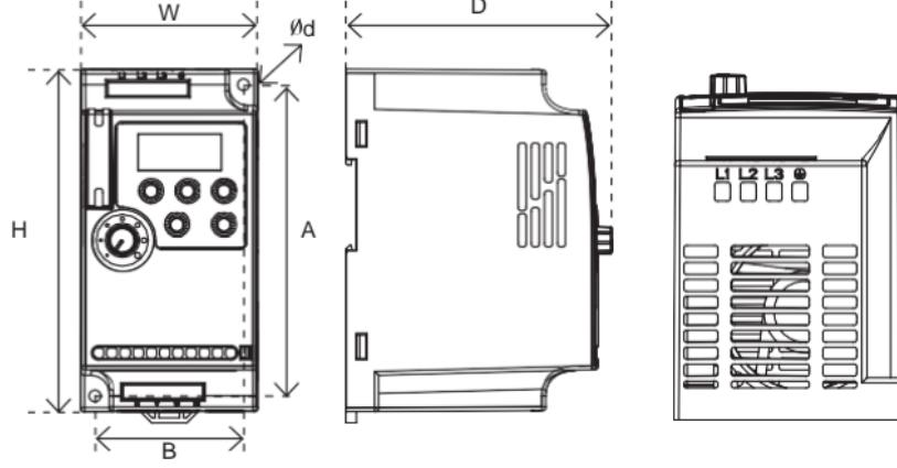
Note: Support for standard 35mm rail mounting(below 5.5kW) Unit:mm
